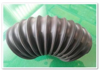
Structure: Outer bore of TPR (thermoplastic rubber); PP-coated spring steel spiral; welded to outer bore.
