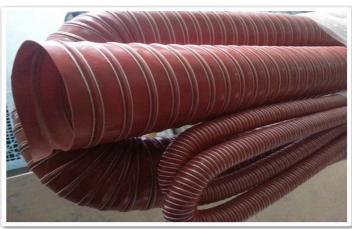
**Structure:** Wall made of 2 ply glassfibre reinforced Silicone; copper plated spring steel spiral embedded into wall, on the outside reinforced with two additional glassfibre cords
